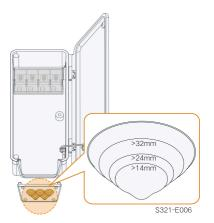
step 5 Lead the cable through the sealing ring and secure the screws on the bottom sealing plate.
